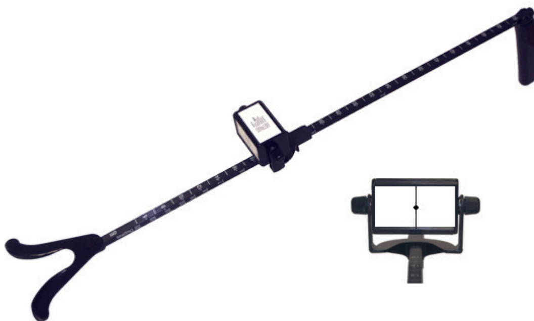
Figure 3. RAF (Royal Air Force) Rule and inset detail of near target block with vertical line and central dot for convergence fixation used by the author to accurately quantify near point of convergence (Modified image from Sussex International, UK, used with permission).
